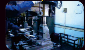
10. Drilling on the as casting
